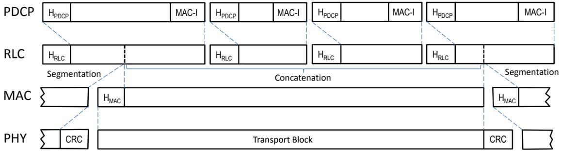
Figure 3: Data flow through protocol layers of LTE;  $H_X$  stands for the header of layer  $X$ .
