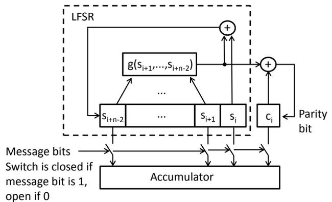
**Figure 1:** The computation of the hash function  $h_{p,s}(M)$  for a message  $M$ .
