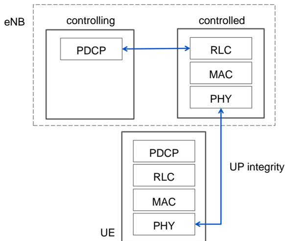
Figure 2: Assumed protocol and security architecture for 5G user plane (UP).
